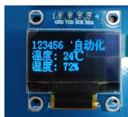
Figure 17. Display module test results
