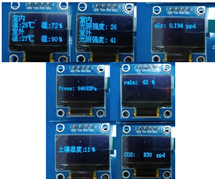
Figure 18. Data acquisition module test results
